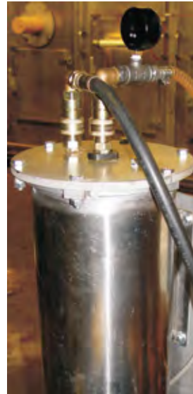
Oil dewatering filter
