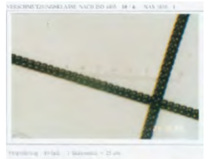
Filter Membrane pore size 0.8 \mu\text{m} after filtration of electrostatic cleaned oil
