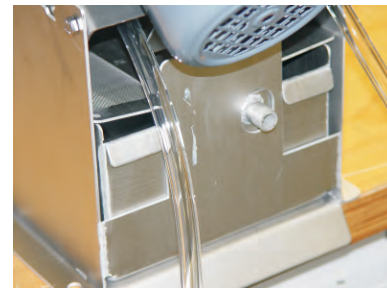
Oil skimmer 1U with decanter tank
