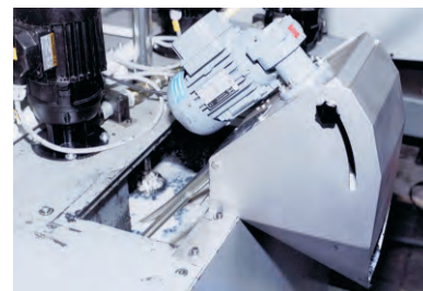
Oil skimmer 1U with open drain
