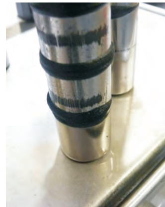
Finest debris collected on magnetic filter rod
