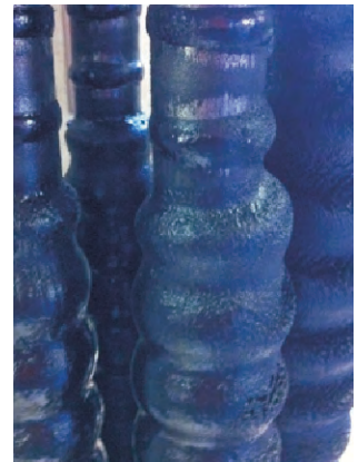
Ferritic particles on magnetic filter rods
