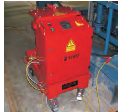
Electrostatic oil cleaner model D4 connected with hydraulic tank of injection molding machine
