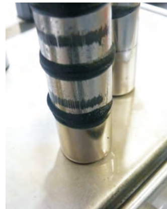
Finest debris collected on magnetic filter rod
