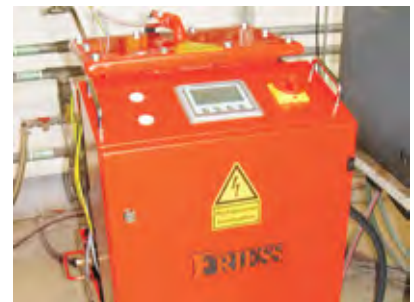
electrostatic oil cleaner model D8 connected with hydraulic tank of injection molding machine
