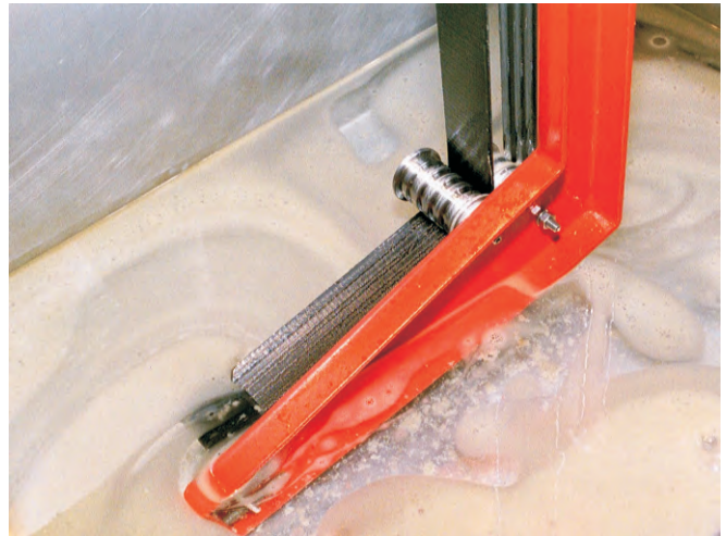
Floating oil is attracted towards the oil skimmer
