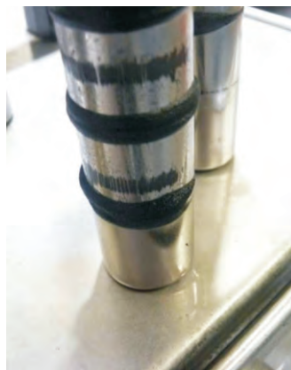
Finest debris collected on magnetic filter rod
