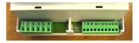
1 - 2: Power Supply (24VAC\* or 115VAC\* or 230VAC\*). \* See instrument's label
