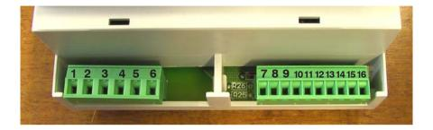
1-2: Power Supply (24VAC\* or 115VAC\* or 230VAC\*). \* See instrument's label
