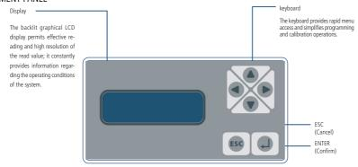
Use the keyboard to select an item or to increase/decrease a value (up, down, right, left). Once the function/item is displayed, press the "enter" key to confirm or press the "ESC" key to cancel or exit from the various screens.
