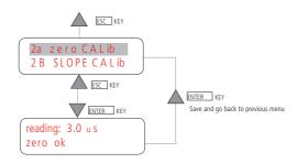
Select "2B SLOPE CALIB" for Slope calibration. Set buffer solution value (0 to 99.9  $\mu$ S). Insert probe into buffer solution. Wait until a stable value and press ENTER to save and exit, or ESC to exit without save. Attention: BUFFER field value must not be 0, otherwise the value will not be saved.
