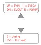
Press: - UP to enable EVIN (Solenoid valve EV1)
