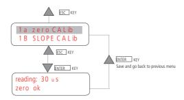
Select "1B SLOPE CALIB" for Slope calibration. Set buffer solution value (0 to 999  $\mu$ S). Insert probe into buffer solution. Wait until a stable value and press ENTER to save and exit, or ESC to exit without save. Attention: BUFFER field value must not be 0, otherwise the value will not be saved.
