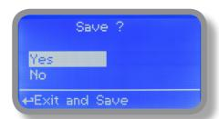
Choose "YES" to save changes. Exit from main menu. Main display will show a countdown for selected output. To stop this countdown go back to "Output Manager" menu and choose "AUTO" as working mode or wait until countdown ends. This function can be used for priming purposes.
