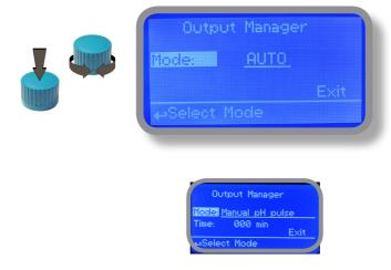
Press wheel to move cursor on "TIME" field. Once here, choose a working time between 0 (disabled) or 199 minutes. Move on "EXIT", then press wheel.
