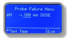
E.g. To set pH pump to stop after time ends and probe doesn't change reading values press wheel, choose maximum time, press wheel move on next field and choose "STOP". Time can be set between 100 and 254 minutes. When satisfied with settings move on exit and press wheel.
