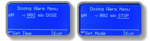
E.g. To set CI pump to stop after time ends and setpoint isn't still reached press wheel, choose maximum time, press wheel move on next field and choose "STOP". Time can be set between 0 and 100 minutes. When satisfied with settings move on exit and press wheel.
