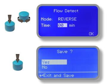
To end procedure move cursor on "OK" and press wheel to proceed to "Save" request screen. Move wheel on "YES" to save or "NO" to discard changes.
