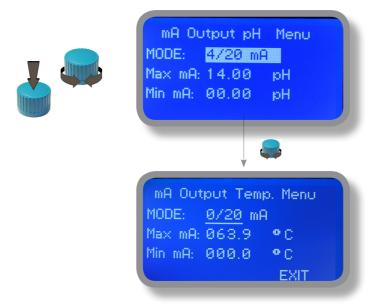
Rotate wheel to move within all 3 channels. Click wheel to selecte parameter and rotate wheel to change it. Click wheel again and rotate wheel to move cursor on next parameter. To end procedure move cursor on "EXIT" and press wheel to proceed to "Save" request screen. Move wheel on "YES" to save or "NO" to discard changes.
