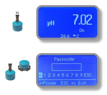
To set a new passcode choose "PARAMETERS" from "Main Menu", move on "New Pcode", click on wheel and enter a four numbers code. Click on "EXIT" and choose "YES" to save request. The new passcode is now ready.
