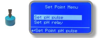
Proportional mode set the instrument to operate using a calculated percentage between two set values that enable or disable the pH pump. To use this mode move cursor on "Working Mode". Press the wheel and select it.
