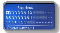
Up to three numbers for sending SMS can be stored into LDSPH memory. SMS recipient will receive an SMS containing instrument ID, NAME and status. Number formats can be stored using international prefix "+", international prefix "00" or local.
